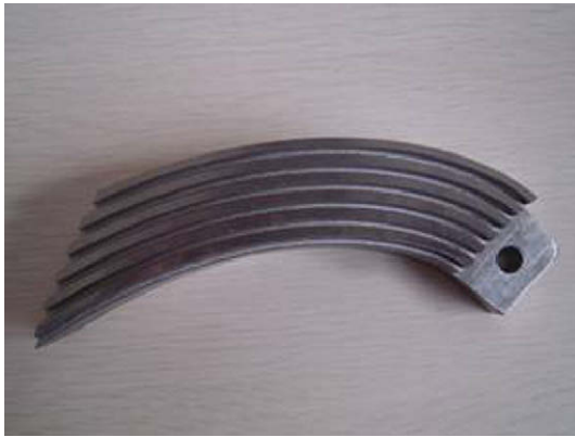
Fig. 3. Involute shaped target ring segment with grooves on the surface.
